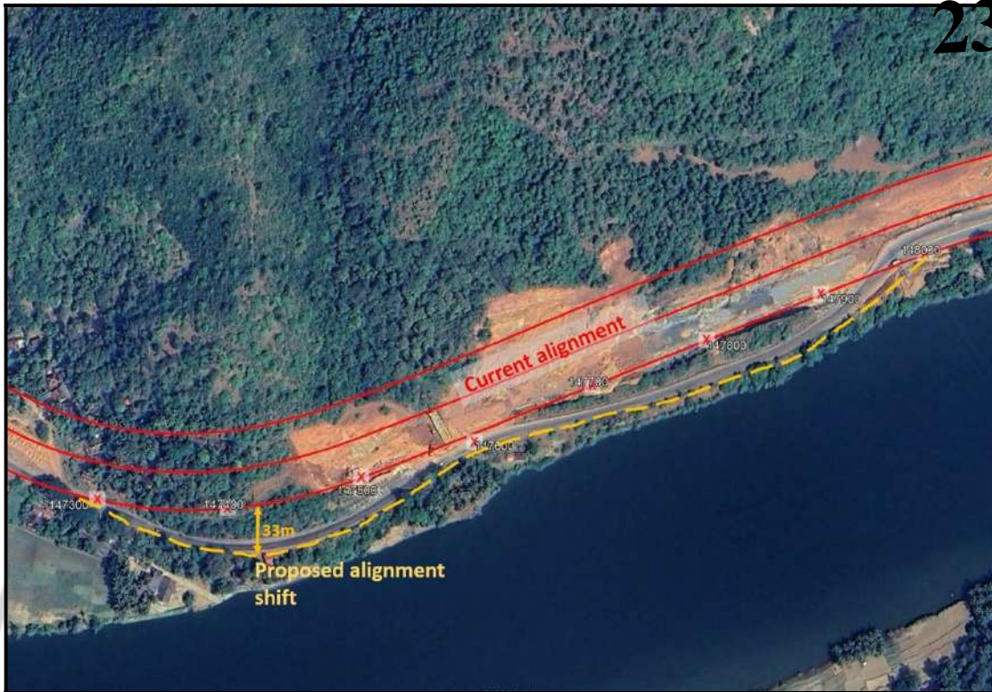
Fig. 2.6: Proposed alignment shift to prevent further slope failures at the Shirur site.
