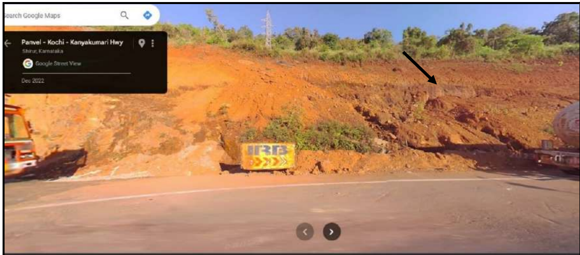
Fig. 1.8: Slump as seen through Google Street View of the Shirur landslide site
