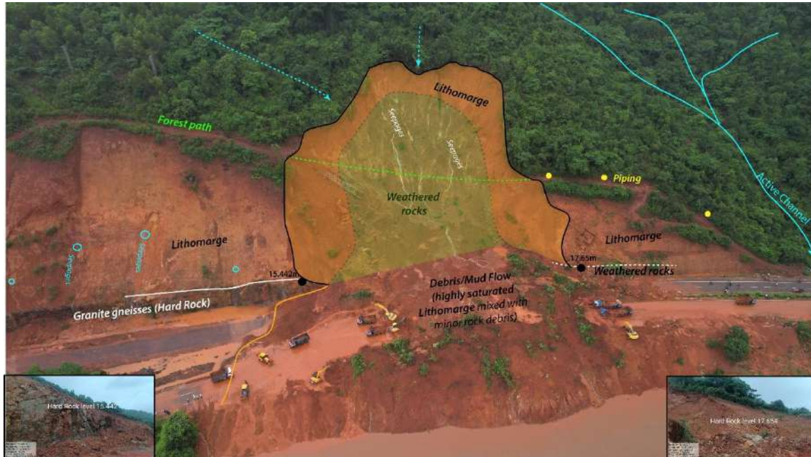
Figure 6: The basic morphological features of the Shirur landslide zone.
