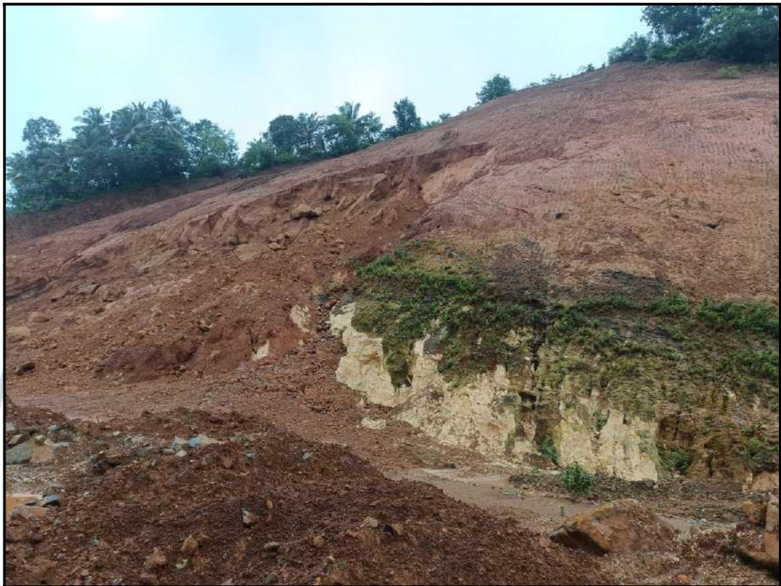
Fig. 2.5: Variability in lithounits near the right flank of the Shirur landslide
